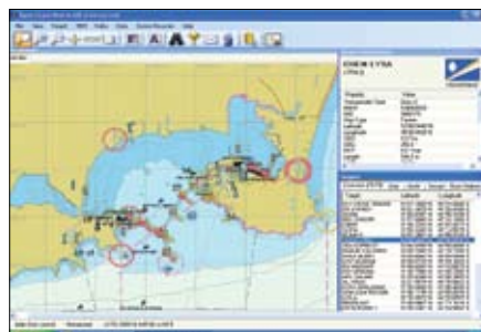
Picture shows AIS targets and information received by AIS equipped Vessels at Port of Aden.
